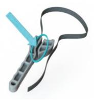
3. Place the strap into the channel with enough slack to fit your sump
