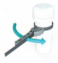
3. Turn wrench to the left/clockwise to loosen
