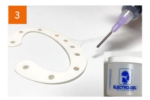
Once there is gel evenly spread over all 10 electrodes, carefully remove the second layer of the adhesive.
