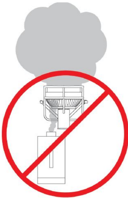
Incorrect ProFan placement in front of fogger/hazer
