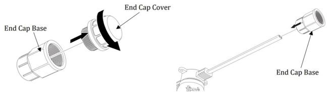
12. Attach the end cap cover onto the end cap base and tighten.
