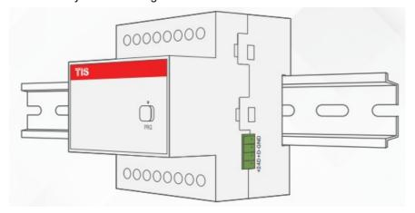
3. Connect a Cat5e TIS network data cable to the TIS-BUS port as per the connection diagram. No need to loop the TIS-bus cable if 2 DIN rail modules are connected together from the side bus train terminal.
