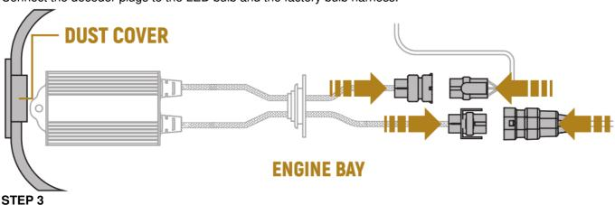
Secure the decoder harness to the inside of the bulb housing. To optimize the heat dissipation of the LED bulb, try to secure the decoder control box away from the LED bulb and the LED driver to avoid excess heat accumulation. Reinstall the dust cover.
