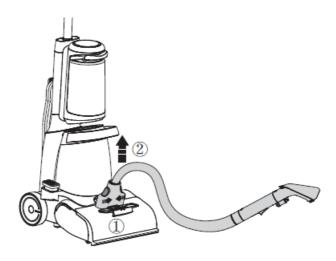
Press the release button to remove the accessory brush.
