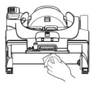
Replace the brush roller by inserting the brush roller end into the right side of the holder, then attach the roller tab to the left side to lock into place.
