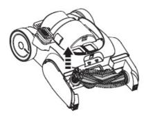
Using the cleaning tool, remove the hair and debris wrapped around the roller and rinse with water. Replace the brush roller back into the accessory holder, and allow it to dry completely before reinstalling.
