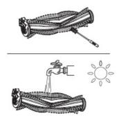
Remove hair and debris from the brush roller chamber and the opening with a tissue or a damp cloth.
