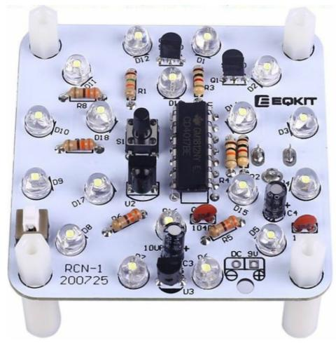
• Step 16: Install 1pcs 9V Battery socket at DC 9V. Note: Red wire connects to ' + '.
