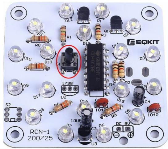
• Step 12: Install 1 pcs VS1738 Infrared receiver at U2.
