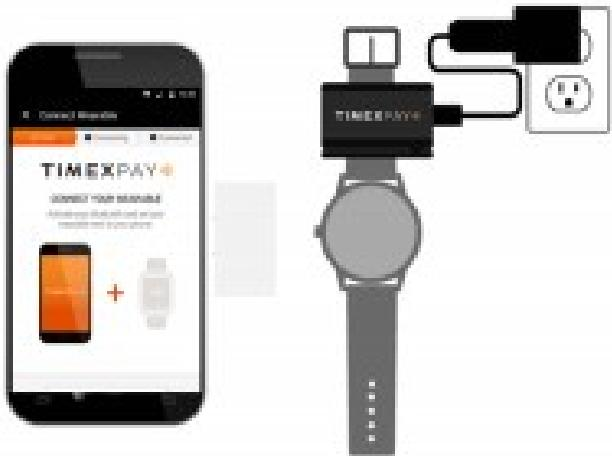
While plugged in and powered on place the UPPU Clip over the indicator symbol on the back of the strap as shown:
