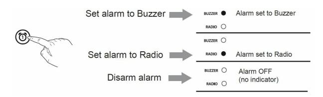
Press and release the Alarm 1 Button repeatedly as needed to cycle to desired alarm mode: Buzzer (default), Radio (last AM or FM station played), or Off (alarm is no longer active). Note that the last radio volume listened to will be the radio alarm volume.
