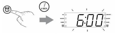
2. Press and release the Hour/ + Button to adjust the HOUR.
