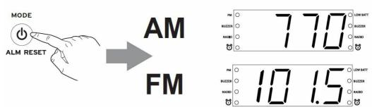
2. Press and release the Hour/ + Button or Minute/ – Button to tune the radio to a desired station. Press and hold to seek the next clear station.
