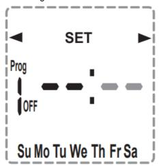
Press the ADV or BOOST buttons to select the Minute that the OFF event will be performed. When finished, press the Prog button.
