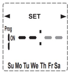
Press the ADV or BOOST buttons to select the Minute that the ON event will be performed. When finished, press the Prog button to proceed to the setting of the OFF event.
