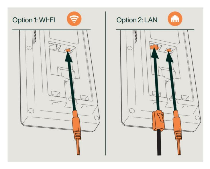
**Option 1:** Wi-Fi for wireless network. Only connect the supplied power adapter to the time clock device. **Option 2:** LAN for wired network. Connect a LAN network cable and the supplied power adapter to the time clock device.
