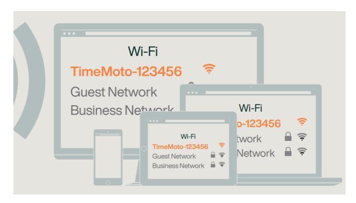
Create a connection between your TimeMoto device and your PC, laptop, tablet or smartphone Use a PC, laptop, tablet or smartphone to scan for available Wi-Fi networks. Then select the temporary network that starts with 'TimeMoto-.....' followed by a six-digit number.
