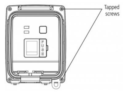
**5.8** Using the back box as a template mark the position for the holes.
