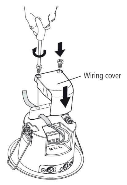
• Push back the locating springs and feed the unit into the ceiling void via the 60mm hole. The locating springs will now fold back and hold the STFM360 in place.
