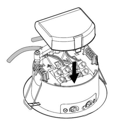
• Push back the locating springs and feed the unit into the ceiling void via the 75mm hole. The locating springs will now fold back and hold the SLFM360N in place.
