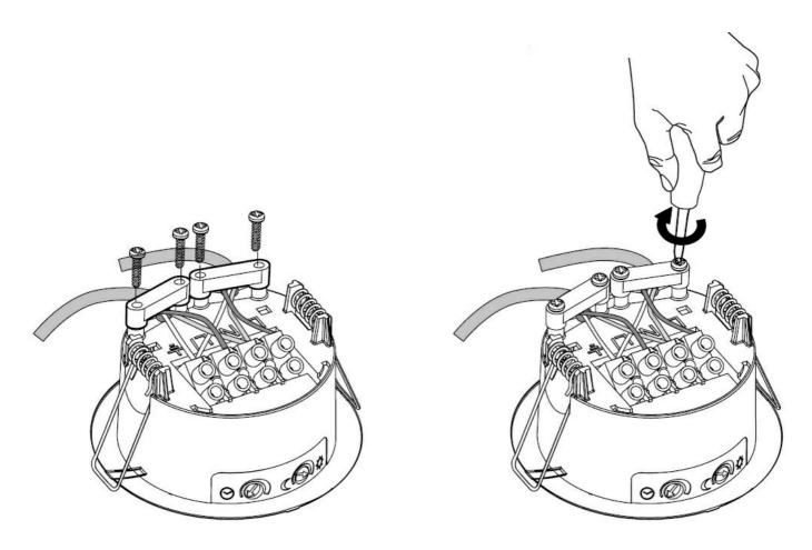
• Reposition the wiring cover onto the sensor and click into place.
