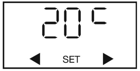
**Note:** The default temperature is 20°C. The temperature set range is 0°C to 35°C.
