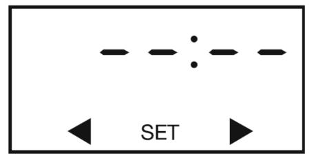
• Use the 'TEMP' button to increase the numeric value, or 'MODE' button to decrease the numeric value. The clock is set in 24 hour format.
