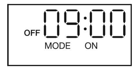
**MODE OFF** – Permanently OFF: The output will be OFF, irrespective of the set temperature.
