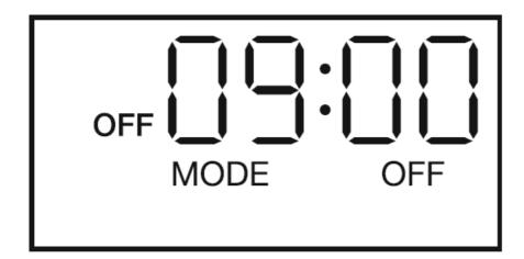
**MODE T** – Timed mode: The output will be controlled by the set temperature, between the programmed ON and OFF times. There is only one set temperature and this cannot be set differently for individual timed periods.
