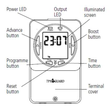
This time switch is an easy to use digital timer, designed for wall mounting. It can control outputs of up to 16A which makes it suitable for domestic immersion heaters.
