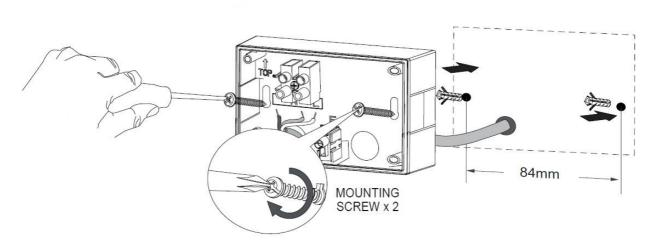
• The mains supply cable can now be terminated. Please refer to section 8 (Connection Diagram).
