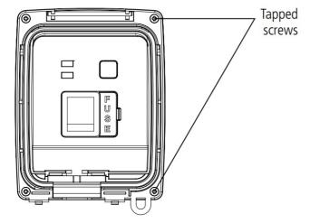
Using the back box as a template mark the position for the holes.
