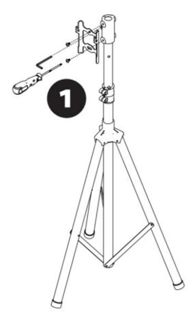
Attach the mounting bracket and tighten the screws.
