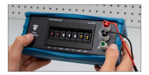
Before use it is recommended that all the digit thumbwheels are rotated completely 2 times. This will ensure the
