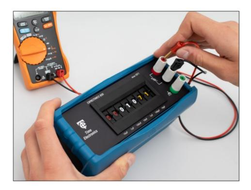
Connection to the decade box is via 4 mm safety terminal posts, using 4 mm shrouded or standard plugs. Alternatively, crocodile clips or stripped wire connections can be used. Whatever method is used, the connection must be tight to the terminal posts to avoid introducing unwanted instability to the capacitance reading. The red and black active terminals connect to the capacitance elements, and the green terminal is connected to the case for screening purposes.
