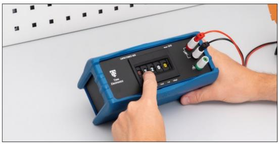
Before use it is recommended that all the digit thumbwheels are rotated completely 2 times. This will ensure the contacts are self-cleaned. This is particularly beneficial if the decade box has not been used for a long time. The 1070 features colour-coded digits to help provide a clear indication of the set values.
