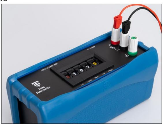
Connection to the decade box is via 4 mm safety terminal posts, using 4 mm shrouded or standard plugs. Alternatively, crocodile clips or stripped wire connections can be used.
