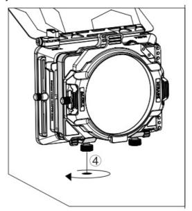
• Mount 2 the variable ND and 3 the matte box body. Tighten the tie down screws.
