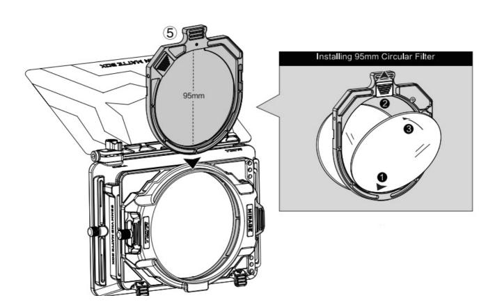
• Pull the locking toggle to release the filter holder.
