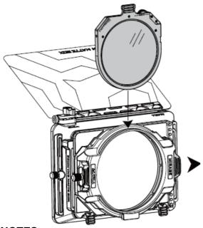
Inserting the 95mm variable ND filter tray.
