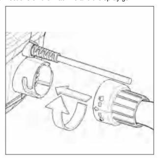
2. Unscrew the container from the spray gun. Align suction tube. The container contents are to be sprayed out almost completely. When spraying horizontal surfaces, turn suction tube forward (A). When spraying objects overhead, turn suction tube back (B).
