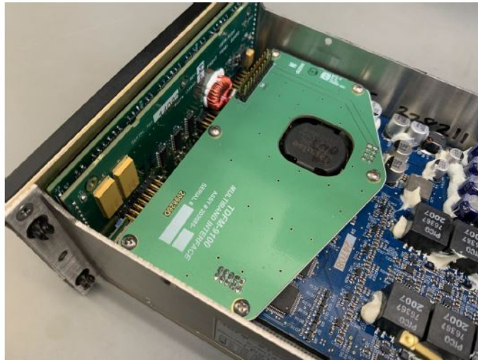
Install 6 screws with lock washers.
