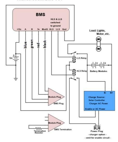
Build up the pack, attach power interconnects and verify power output, then connect module plugs between modules until all but the end plugs are connected. Connect the BMS Termination and BMS Plug (see below) to the end module connectors. Next, refer to the diagram below and complete the BMS wiring per the actual system requirements.
