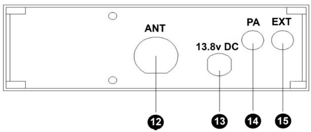
Antenna connector. Refer to the section INSTALLATION OF THE ANTENNA.
