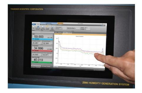
**Temperature Control:** The 2900 humidity generation system incorporates a water/glycol jacked test chamber for extremely stable temperature control. The system uses PID (proportional-integral-derivative) algorithms to control the temperature of the chamber fluid as it is pumped around the test chamber and through the saturator at the rate of approximately 14 gallons per minute by a magnetically coupled centrifugal pump.
