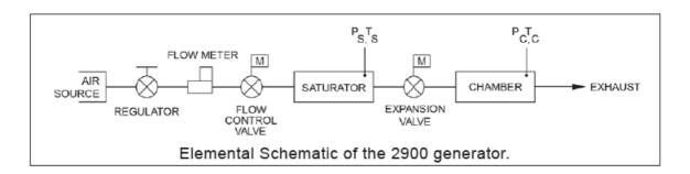
**Pressure and Flow Control:** Pressure control and mass flow control are accomplished through computer actuation of electromechanical valve assemblies. Saturation pressure and mass flow are measured continuously and controlled using PID algorithms similar to those employed in temperature control.
