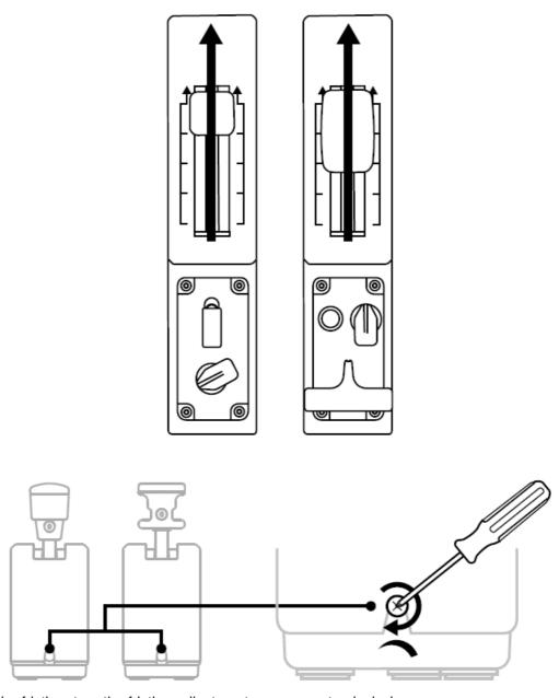
3. To decrease the friction, turn the friction adjustment screw counterclockwise.
