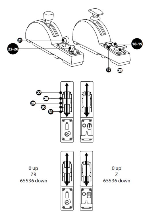
The TCA Quadrant Add-On Airbus Edition modules feature mechanical selectors allowing you to disable the detents/notches on each axis. Doing so allows you to have smooth axes, while maintaining virtual buttons 27 through 31 on the speed brake module.
