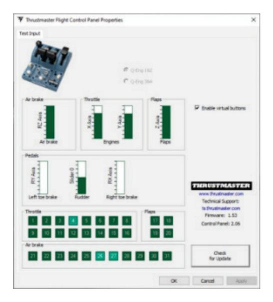
**Enable virtual buttons:** This feature lets you enable or disable the virtual buttons available on the axes for the throttle quadrant, and the speed brake module. Click **Apply** once you have selected the mode you want to use.
