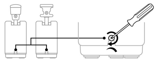
3. To decrease the friction, turn the friction adjustment screw counterclockwise.
