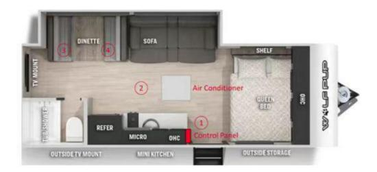
The module is installed in the WFCO smart power control system position 1 in the following figure. The installation requirement is SMT mount. The antenna is in the picture position 2, and the distance between the antenna and the human body is greater than 20cm. The device is only used indoors. Modules are only used by applicants to install into our own products.
