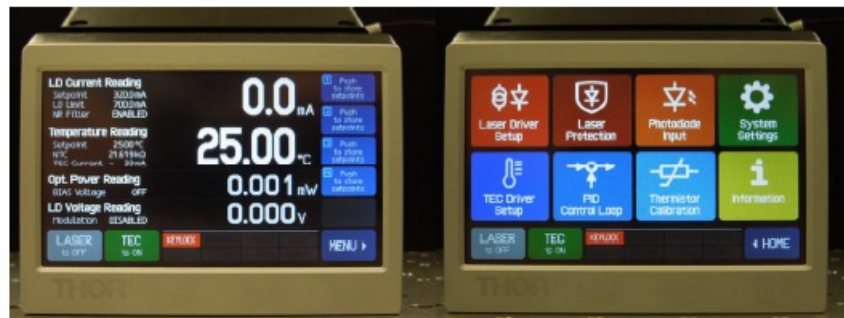
Figure 2 Laser Controller Screen at Start-Up and When Entering 'Menu'
