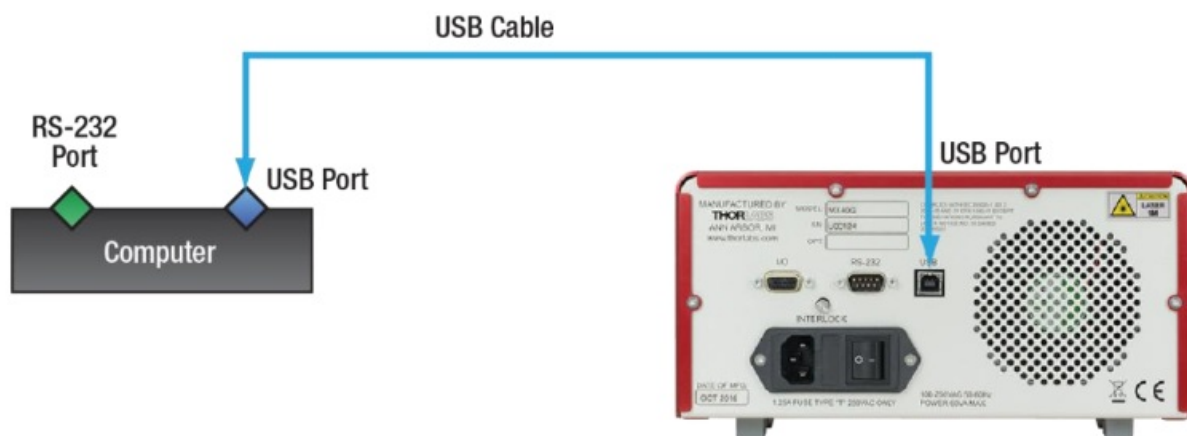
Figure 2 Connecting the Computer and Instrument via the USB Ports
