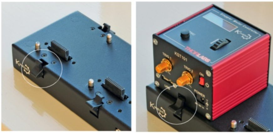
Fig. 2.9 Fitting A K-Cube Driver Unit
