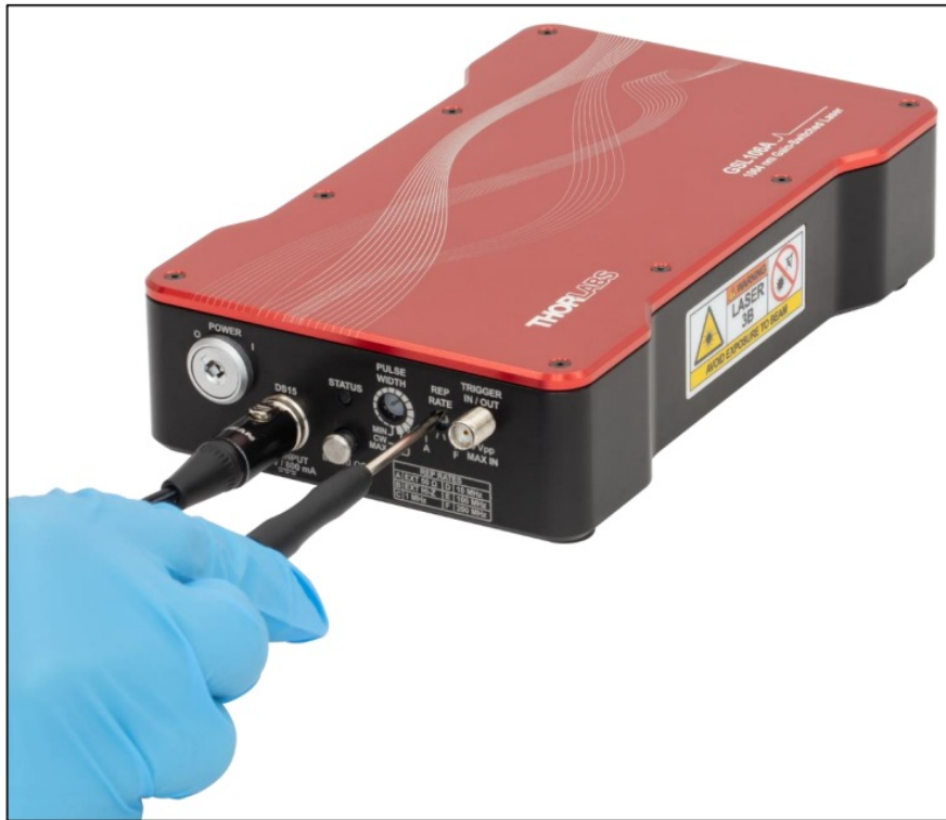
Figure 6 Pulse width and repetition rate controls are adjusted with the included 2.5 mm flathead screwdriver.
