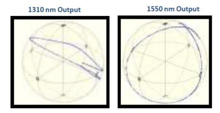
• All three paddles started in the fixed, vertical position and then each paddle was articulated through its full travel range while the other two remained in their starting, vertical positions.
