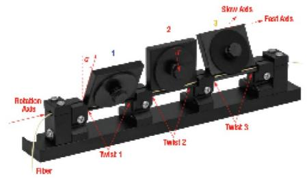
**Bending** the fiber around in a number of loops (N) about the coil diameter (D) creates bend-induced retardation:
