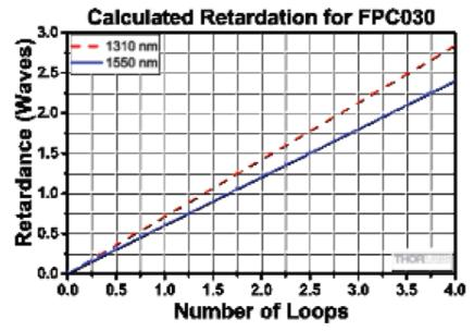
Theoretical retardation vs. the number of loops for 1310 nm and 1550 nm.
