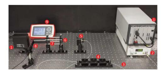
1. 1000 – 1250 nm Polarimeter: PAX5710IR2-T
