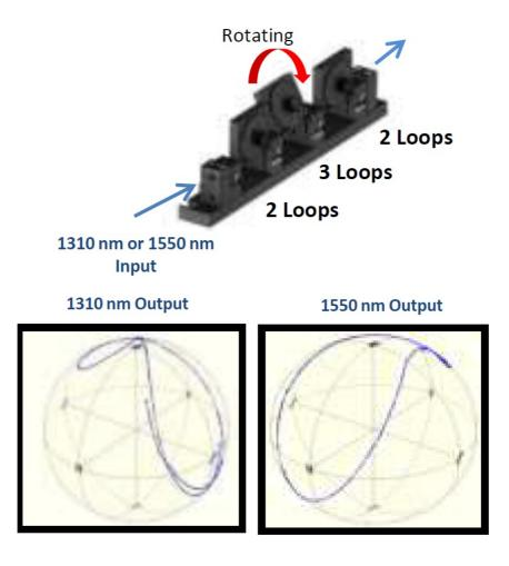
• The 2-loop paddles provided displacement predominantly in the vertical direction (between the circular polarization poles).
