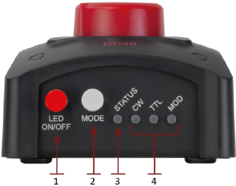
Figure 3 Front Panel of the DC40 LED Driver
