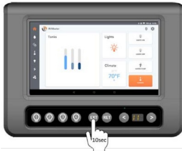
Figure 7: Navigate to 'PA' and press and hold EXT for 10 seconds to clear the RVMasterNode memory
