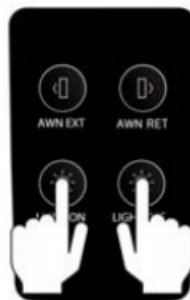
Figure 25: Press any two buttons on the RVMasterSwitch
