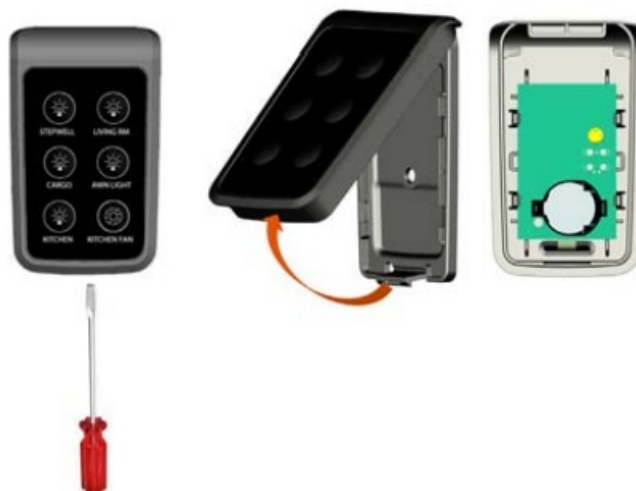
Figure 21: Accessing the battery in the RVMasterSwitch
