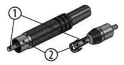
Drawing and table indicate the pin assignment of an RCA plug.
