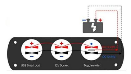
The underside of this car USB charger is marked with "+" and "." for plus and minus poles. Connect "+" to the positive pole of the battery. "-" to the negative pole.
