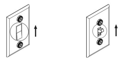
(7) Place Smart Switch over existing switch. Test the switch by pressing the button to turn on and off. Adjust the spacers to ensure proper engagement between the Smart Switch and wall switch.
