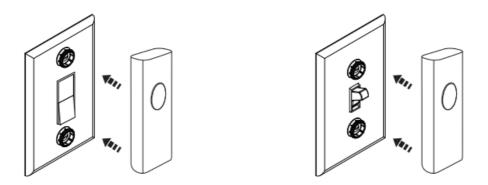
Optional – For rocker switch, place protective film over paddle, as shown.
