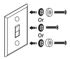
In most case, you need to combine fixator with thin rubber ring. However, you can also use fixator only or combine fixator with thick rubber ring to adjust the thickness of attachment assembly.
