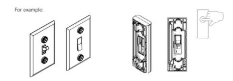
When switch lever or switch board is up, make sure the Smart Switch clip position is up, you can manually quick press the switch button to adjust the clip position if necessary.
