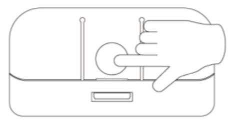
3. Long press the inside button of the sensor to get it in pairing mode. Release the hold until you see the red LED turn on. After you release the hold, LED will change to a blue fast blinking that indicates the Door Sensor is now ready to be set up.
