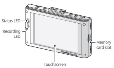
Gently touch the screen to make inputs on the touchscreen. The screen may be damaged if you apply excessive force to the screen or if you touch the screen with a sharp object.
