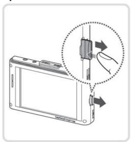
Before removing the memory card, ensure that the product is turned off. Gently push the bottom of the memory card with your fingernail to release it, and then remove it from the product. To insert the memory card into the memory card slot, ensure that the metal contacts on the memory card are facing toward the lens of the product, and insert it into the slot until you hear a click.
