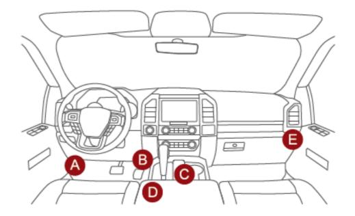
**Note**: Tire pressure programming, learning and OBD diagnostic functions can be performed by connecting the DLC port. Normally, the OBD port is located under the instrument panel, above the pedal on the driver's side. The OBD port is normally located under the instrument panel, above the driver's side pedal. The five locations shown in the diagram are common OBDII port location
