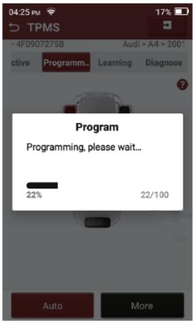
The programming process usually takes 1 minute, the end of the process will prompt you with the programming result, and the sensor data will be displayed on the screen when it is complete.
