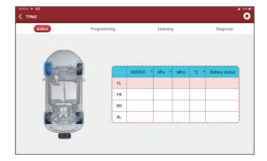
This function allows users to activate the TPMS sensor to view sensor data such as sensor ID, tire pressure, tire frequency, tire temperature, and battery condition.
