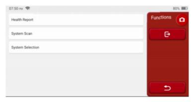
**A. Health Report:** this mode is to quickly check the vehicle and display the vehicle health report (it's available only when the diagnosis software support this function).
