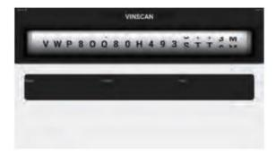
If the device failed to access the VIN information, please use "Diagnosis". At this point, you need to manually input the VIN code to gain the car information.
