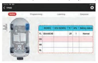
• **Programming**: to program sensor data to a new THINKCAR sensor, so as to replace a sensor that is in low battery and does not function properly. There are three sensor programming methods available: Automatic, manual, and via activation replication.
