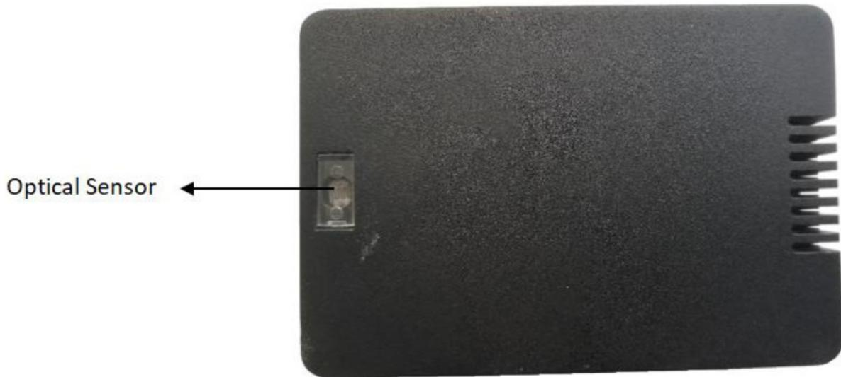
The TMY07 has a built-in optical sensor. When the device is removed after installation and the sensor is exposed to light, it will be activated immediately and the TMY07 will send a “DEVICE\_REMOVED” alarm message to the Platform, together with the current location data.
